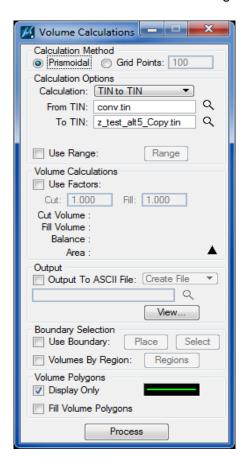
Navigate and Load the two .tin files (the proposed surface .tin from Roadway Designer and the XML generated .tin) for comparison.
