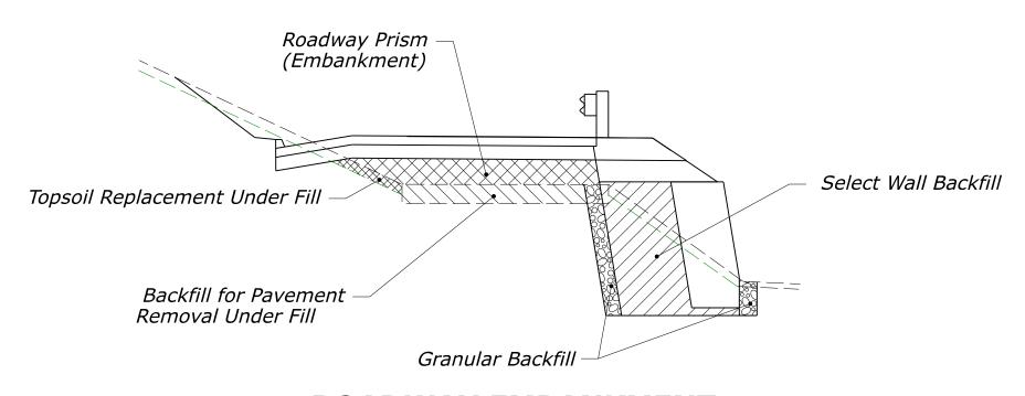
ROADWAY EMBANKMENT GABION FACED MSE
