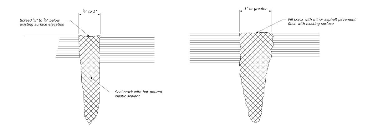
**CRACK SEALING DETAILS**
