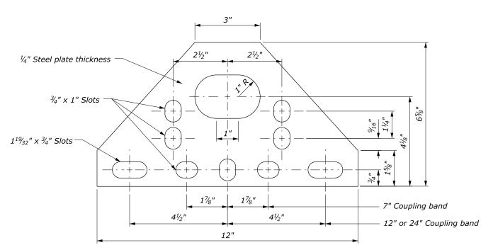
Measure length of coupling band parallel to the centerline of the pipe
